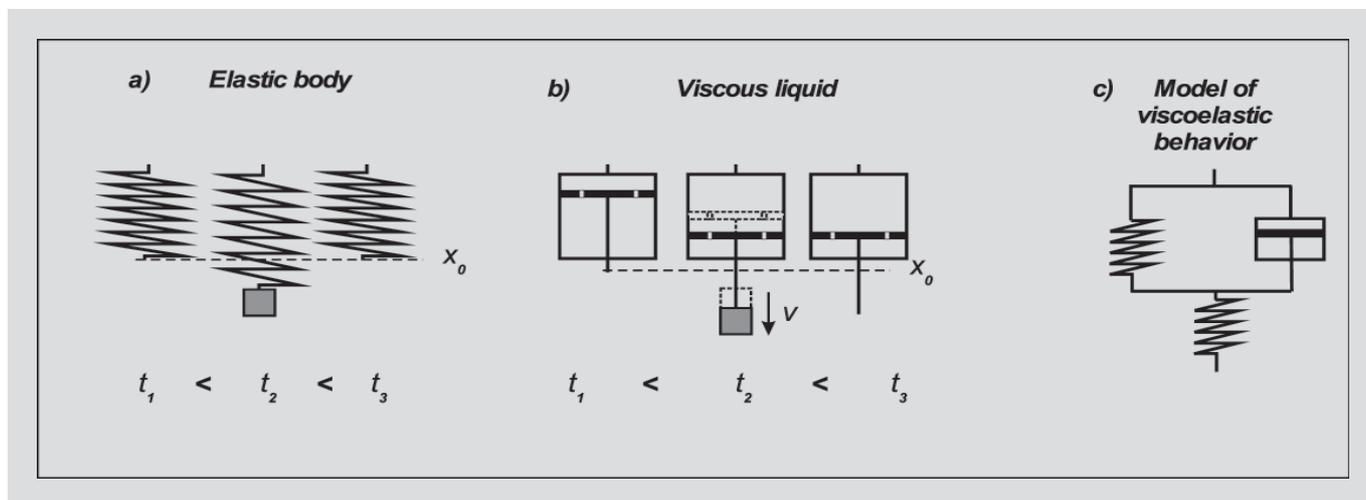
Fig. 1. Models illustrating the mechanical behavior of materials.  $t_1$ ,  $t_2$  and  $t_3$  are the times before, during and after the load was applied,  $x_0$  is the initial length and  $v$  is a constant rate.
