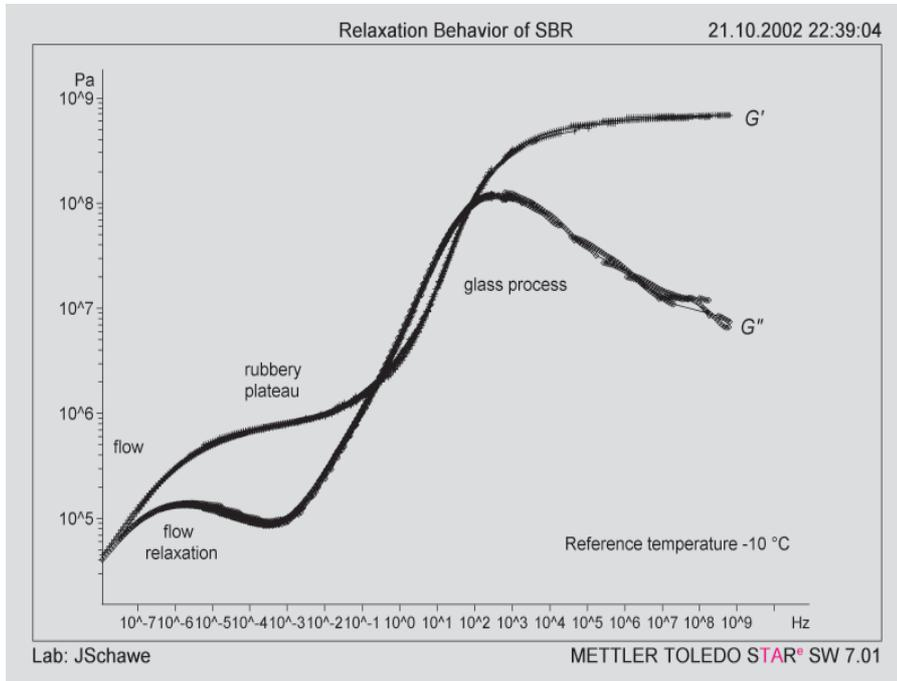
Fig. 4. Storage and loss modulus of SBR at -10 °C.
