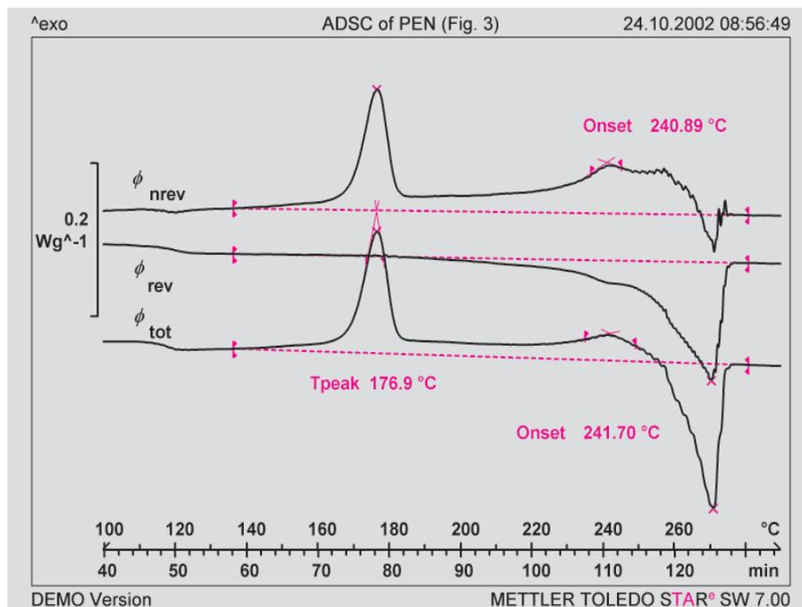
Fig. 3. The total heat flow,  $\phi_{tot}$ , reversing heat flow,  $\phi_{rev}$ , and non-reversing heat flow,  $\phi_{nrev}$ , curves of a PEN film obtained from ADSC measurements with an underlying heating rate of 2 K/min, an amplitude of 0.318 K and a period of 60 s. The temperature maximum of the crystallization peak is given for the total and non-reversing heat flow curves.
