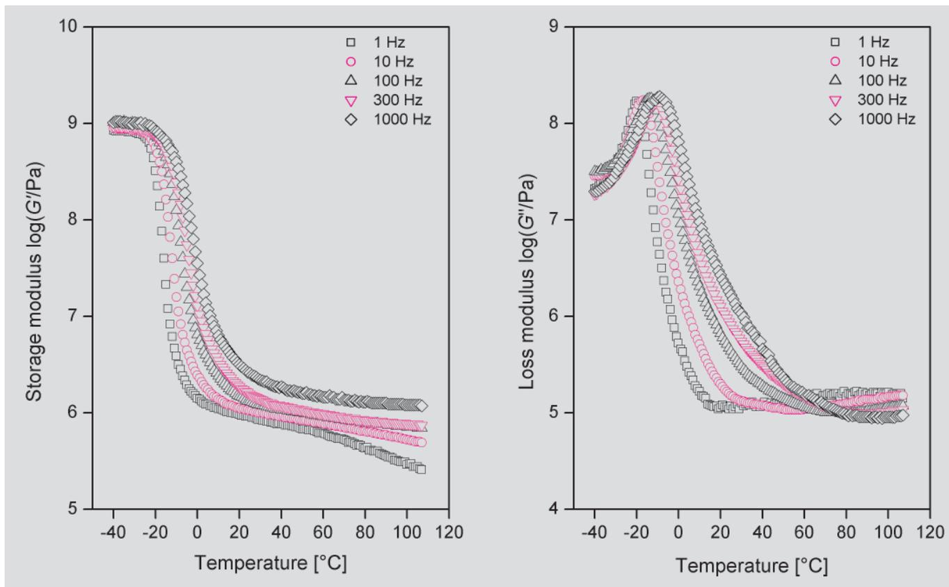
Fig. 1. Temperature-dependent modulus measurements of VSL5025-0 (L-SBR with contents of 25% styrene and 50% vinyl) at different frequencies.
