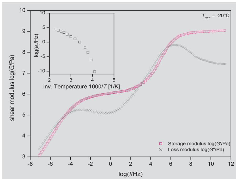
Fig. 2. The master curve of VSL5025-0 constructed from frequency-dependent measurements at a reference temperature of -20 °C, and the shift diagram (upper left).
