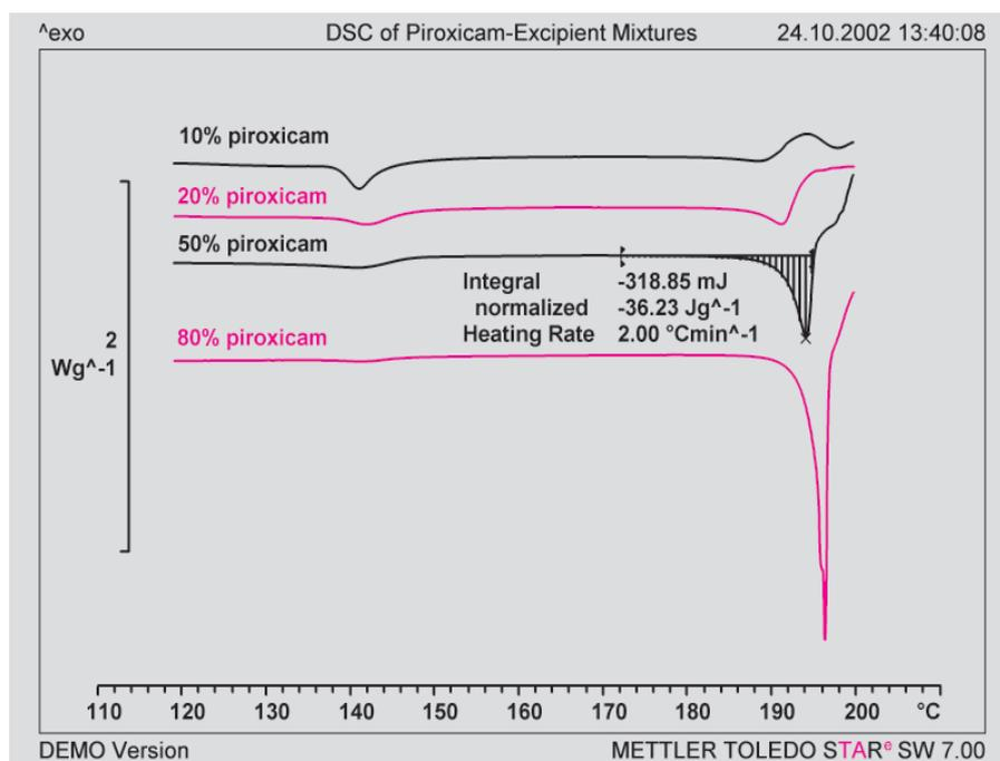
Fig. 2. DSC curves of mixtures with different contents of piroxicam; heating rate 2 K/min, sample weight 8 to 12 mg. Reactions of individual excipients occur below 160  $^{\circ}$ C. The piroxicam melting peak appears in the range 185 to 200  $^{\circ}$ C and is followed by immediate exothermic decomposition. The baseline type "horizontal from left" was therefore chosen to calculate the peak area (see example with 50% piroxicam).
