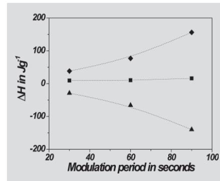
Fig. 2. Effect of the period on the values of  $\Delta H$  obtained by integration of the total heat flow (■), the reversing heat flow (◆) and the non-reversing heat flow (▲). The underlying heating rate was 2 K/min. The amplitude was chosen so that  $\beta = 0$ , i.e. 0.159 K for 30 s, 0.318 K for 60 s, and 0.477 K for 90 s. These results were obtained with a PET film.
