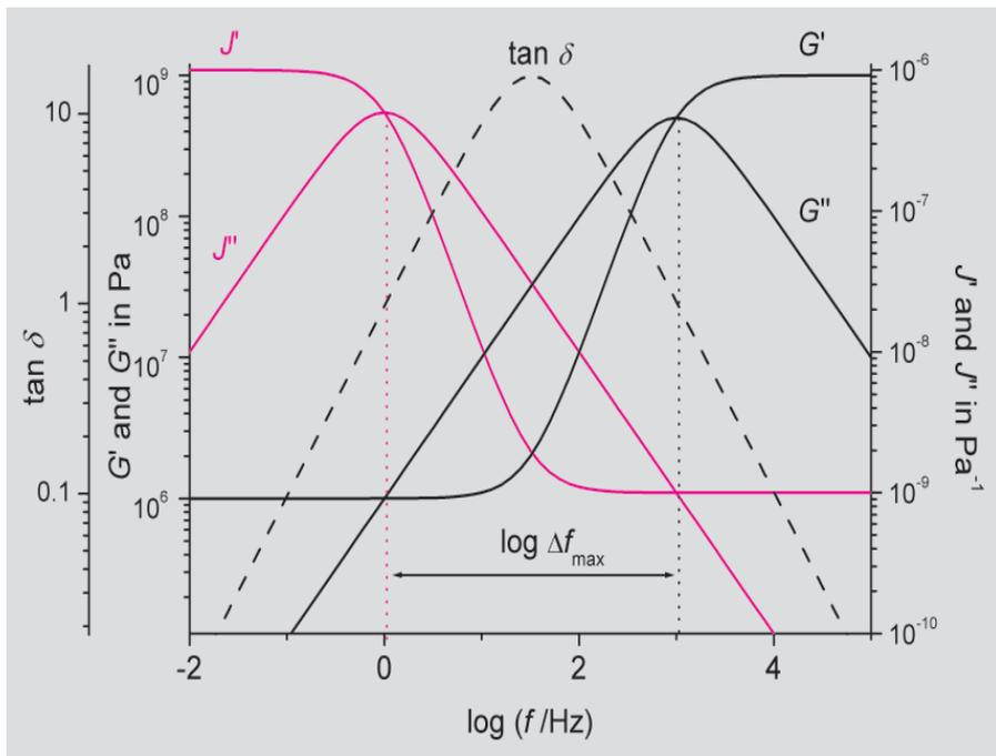
Fig. 2. Basic curve shapes of moduli, compliances and  $\tan \delta$  as a function of frequency.
