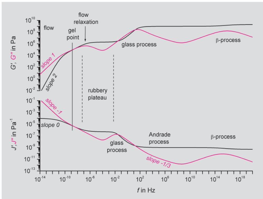
Fig. 3. Schematic curves of moduli and compliances for a viscoelastic material.
