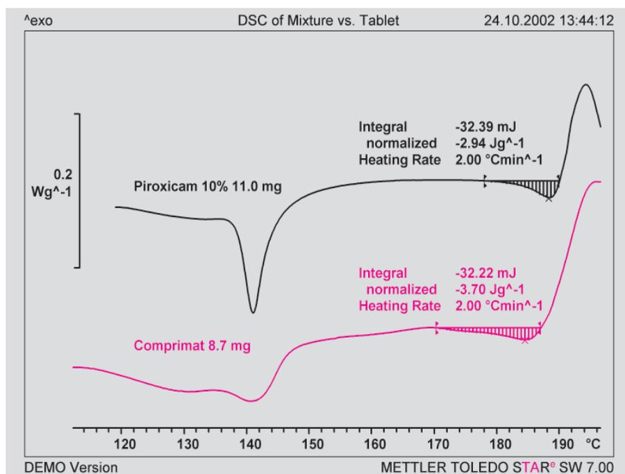
Fig. 4. Below 160 °C, in the region of the excipients peak (moisture, water of crystallization), the DSC curve of the tablet (Comprimat 8.7 mg) is somewhat different to the curve of the sample with the same piroxicam content (10%) obtained by grinding piroxicam with the excipients. The curves are, however, very similar in the region in which the piroxicam melts.
