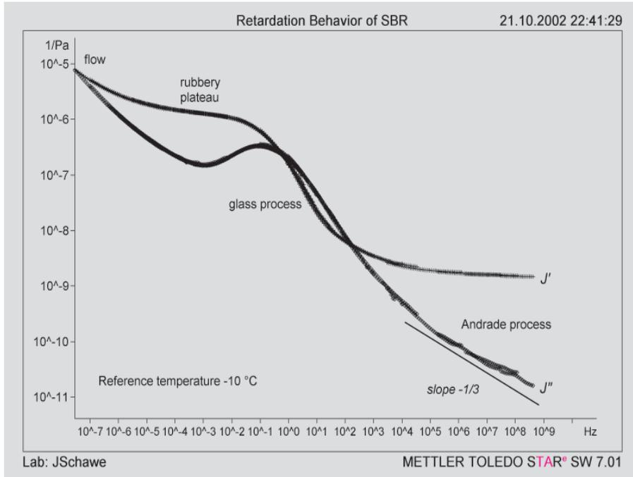
Fig. 5. Storage and loss compliance of SBR at -10 °C.
