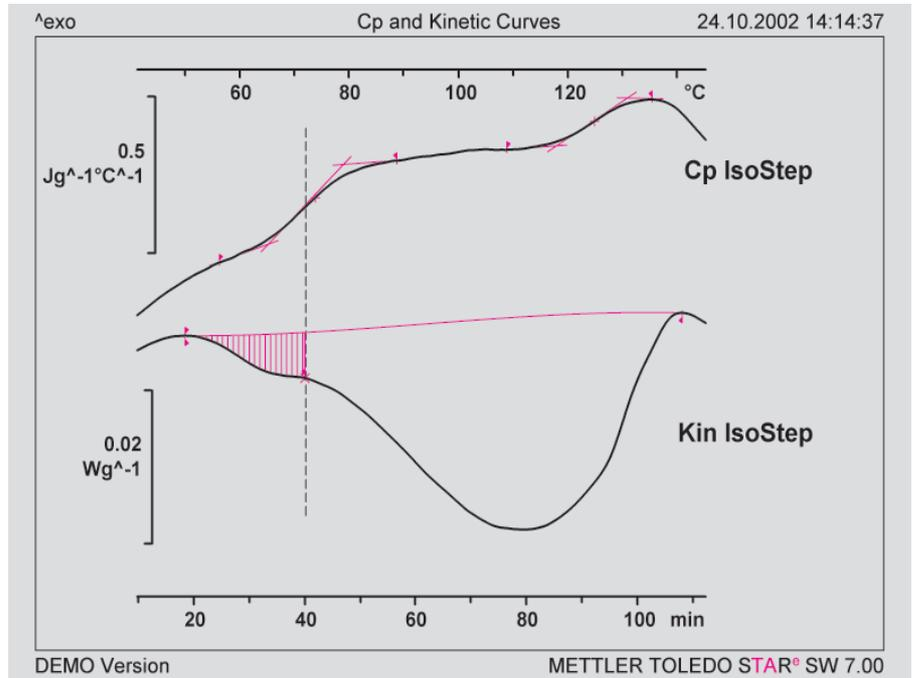
Fig. 2. Specific heat capacity and non-reversing (kinetic) curves as a function of the temperature or measurement time, calculated from the measurement in Figure 1. The hatched area shows the amount of water vaporized up to the glass transition temperature.
