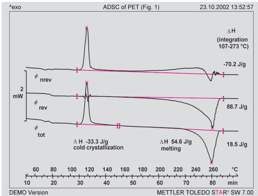
Fig. 1. The total heat flow,  $\phi_{tot}$ , reversing heat flow,  $\phi_{rev}$ , and non-reversing heat flow,  $\phi_{nrev}$ , curves of a PET film obtained from ADSC measurements with an underlying heating rate of 3 K/min, an amplitude of 0.2 K and a period of 50 s. The values of the integrals between the beginning of cold crystallization (107 °C) and the end of melting (273 °C) are shown for the different heat flow curves.
