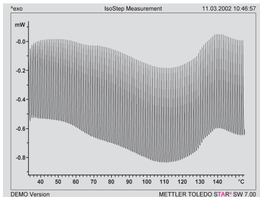
Fig. 1. IsoStep™ measurement as a function of the temperature of a sample that had been preheated at 80 °C for 20 min.
