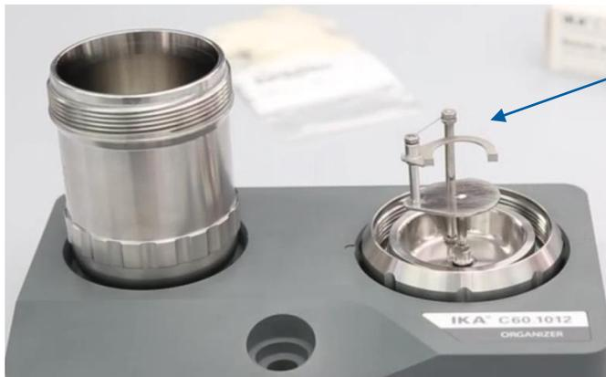
The sample preparation is easy, and can be done without having to use a separate stand, due to turned around electrodes and crucible holder of the decomposition vessel
