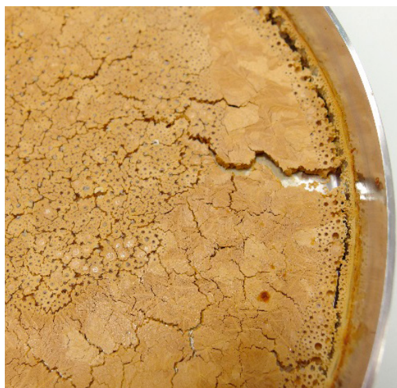
Figure 2: Dried TGY sample exhibiting a porous structure.
