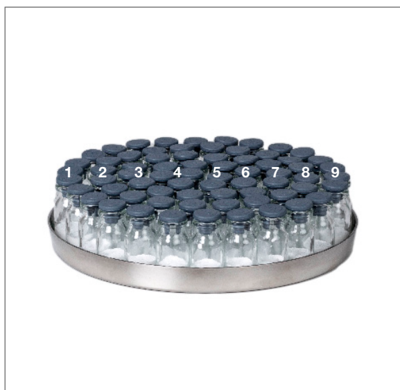
Figure 1: Steel shelf with the freeze dried samples.
