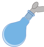
Figure 18: Shell frozen flask with a homogeneous layer of water on the inner wall.
