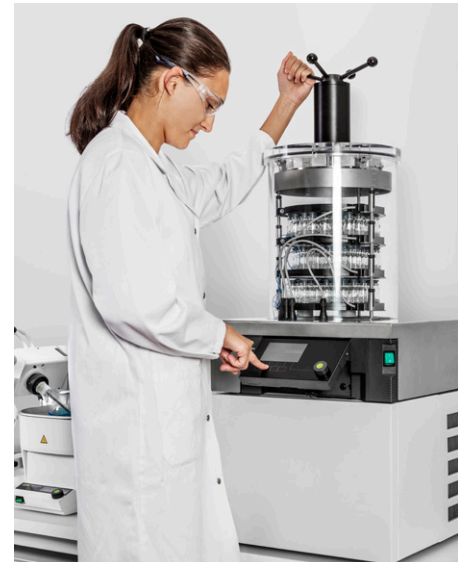
Figure 2: Freeze drying in vial. The system includes stoppering trays and a stoppering top.
