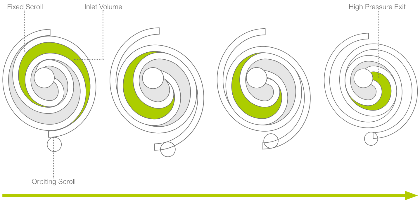
Figure 10: Schematic diagram of a scroll pump
