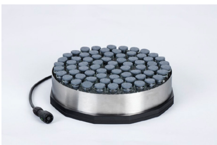
Figure 31: Placing a ferrule on the shelf around the samples will help protect them from radiation
